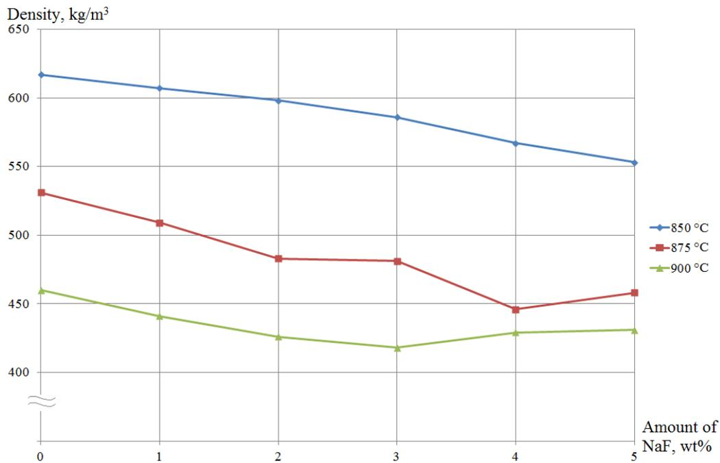
Figure 7. The density change dependence on the ratio of fluxes
