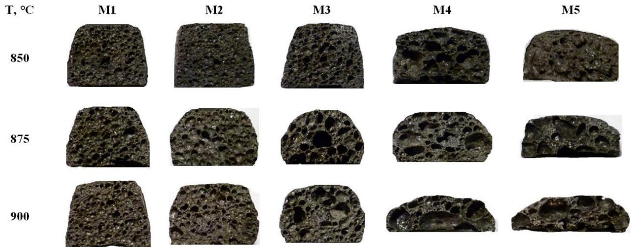
Figure 6. The influence of the fluxes ratio on the foamed slag glass structure
