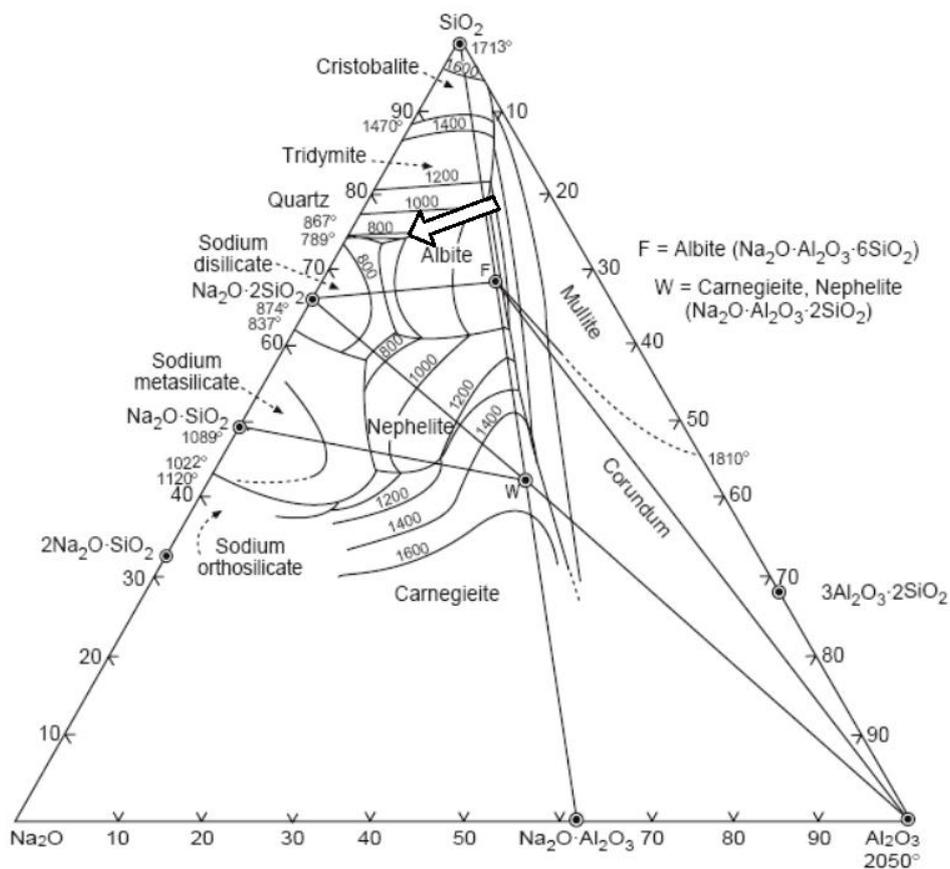
Figure 8. Phase diagram of «Na<sub>2</sub>O-Al<sub>2</sub>O<sub>3</sub>-SiO<sub>2</sub>» system (according to Osborne and Muang)
