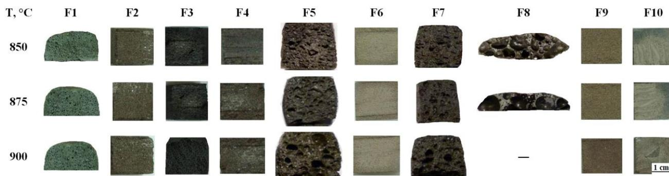
**Figure 5. The influence of the flux type on the foamed slag glass structure**
