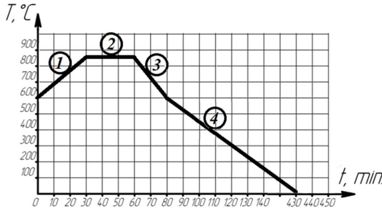
Figure 4. FSG synthesis mode:
