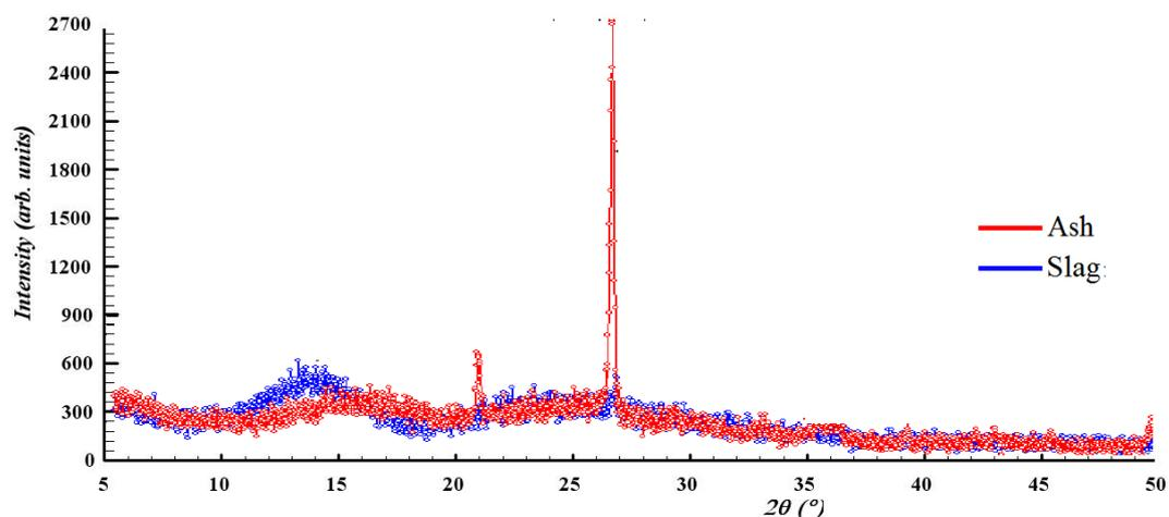
Figure 1. The XRD patterns of ash and slag
